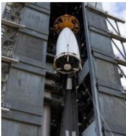
Figure 9-5: Spacecraft During Hoist Operations
