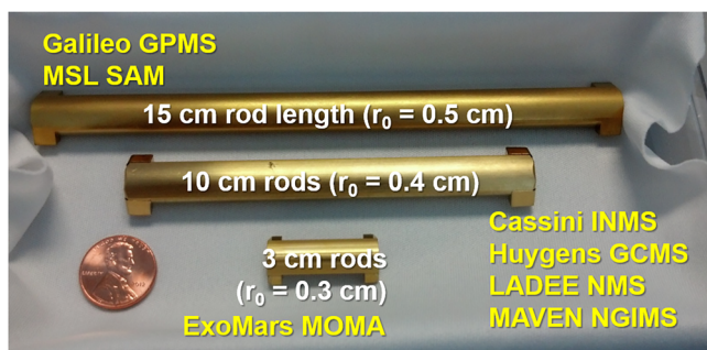
FIGURE 6 Since the Pioneer Venus Orbiter Neutral Mass Spectrometer (ONMS), more recent quadrupole mass spectrometer (QMS) instruments have implemented longer hyperbolic rods in order to expand mass range and maintain or improve mass resolution. The hyperbolic rods manufactured for the Mars Organic Molecule Analyzer (MOMA) linear ion trap, onboard the ExoMars rover, leverage the same mechanical design as heritage QMS systems. Image modified from Arevalo Jr. et al 45
