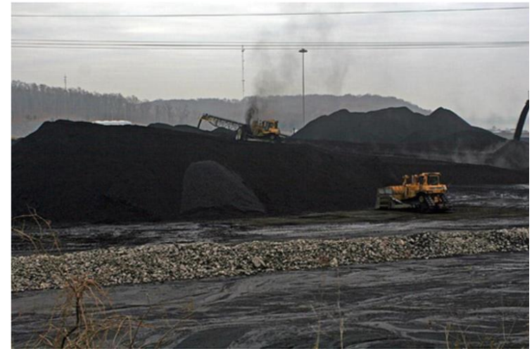
3 days worth of coal supply for a 500 MW plant
