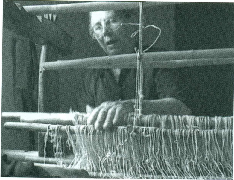
Figure 3 Arremissi: Putting the yarns on the heddle.
