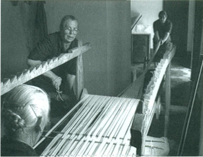
Figure 2 Imboddiai : Winding the warp onto the loom.
