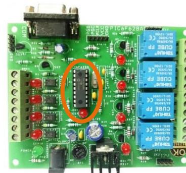
PLC board 4 in 4 out PIC MCU
