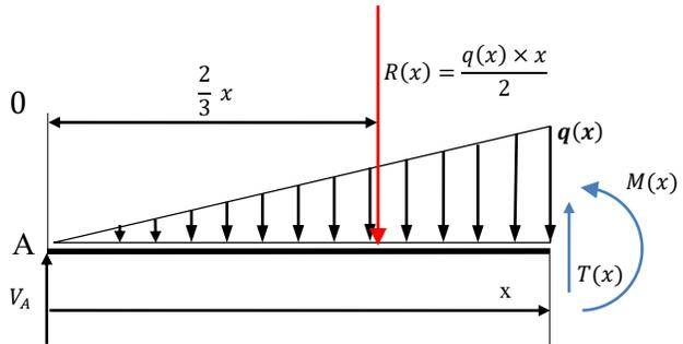
$$M(x) = V_A \times x - R(x) \times \frac{x}{3} = 3333.33 \times x - \frac{q_{max} \times x^2}{2L} \times \frac{x}{3} = 3333.33 \times x - \frac{q_{max} \times x^3}{6L}$$
