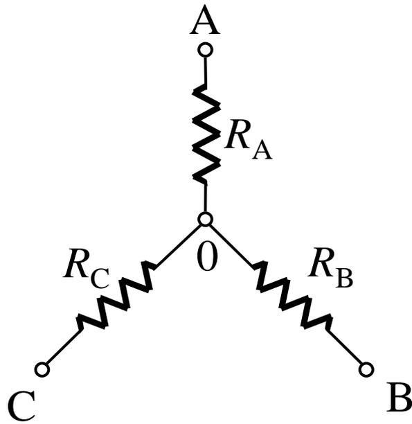
$$\begin{cases} R_A = \frac{R_{AB} R_{CA}}{R_{AB} + R_{BC} + R_{CA}} \\ R_B = \frac{R_{BC} R_{AB}}{R_{AB} + R_{BC} + R_{CA}} \\ R_C = \frac{R_{CA} R_{BC}}{R_{AB} + R_{BC} + R_{CA}} \end{cases}$$
