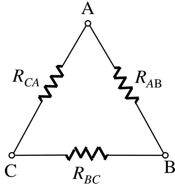
$$\begin{cases} R_{AB} = \frac{R_A R_C + R_B R_C + R_A R_B}{R_C} \\ R_{BC} = \frac{R_A R_C + R_B R_C + R_A R_B}{R_A} \\ R_{CA} = \frac{R_A R_C + R_B R_C + R_A R_B}{R_B} \end{cases}$$
