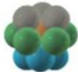
Cubic close-packed (face-centered) crystal structure
