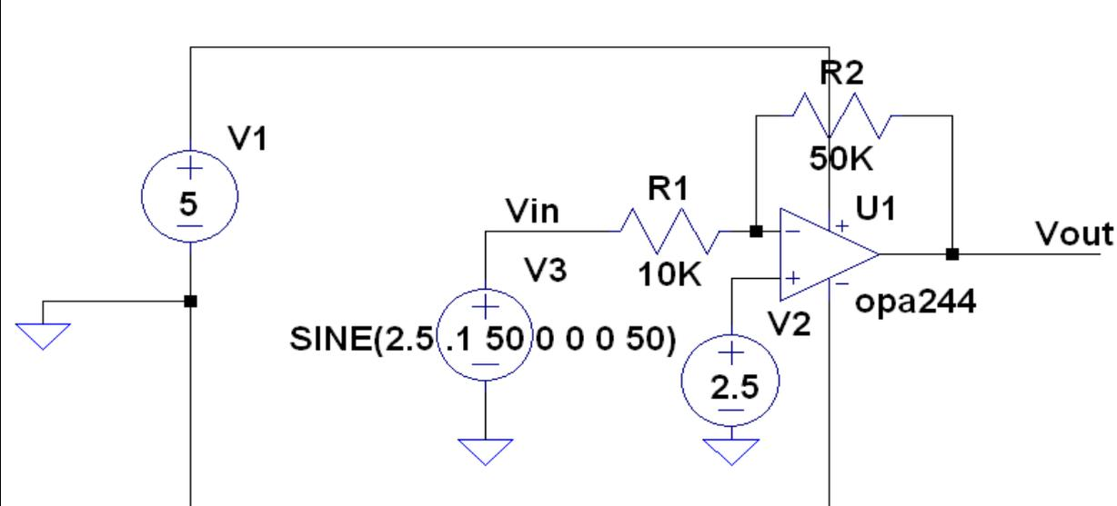
$$V_{out} = V_1 \left( -\frac{R_2}{R_1} \right) + V_2$$
