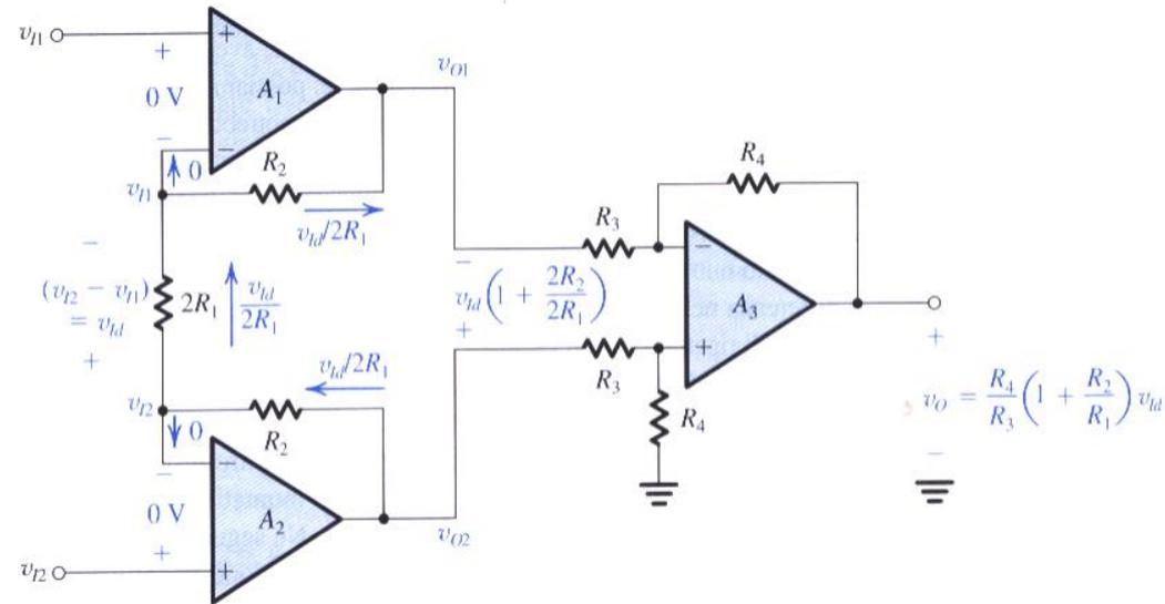
$$v_{O2} - v_{O1} = v_{i2} - v_{i1} + v_{id} \left( \frac{R_2}{R_1} \right)$$
