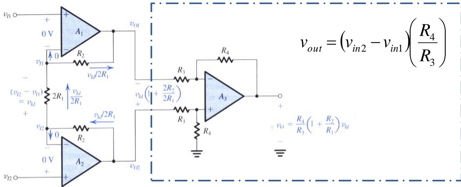
$$v_{O2} - v_{O1} = v_{id} \left( 1 + \frac{R_2}{R_1} \right)$$
