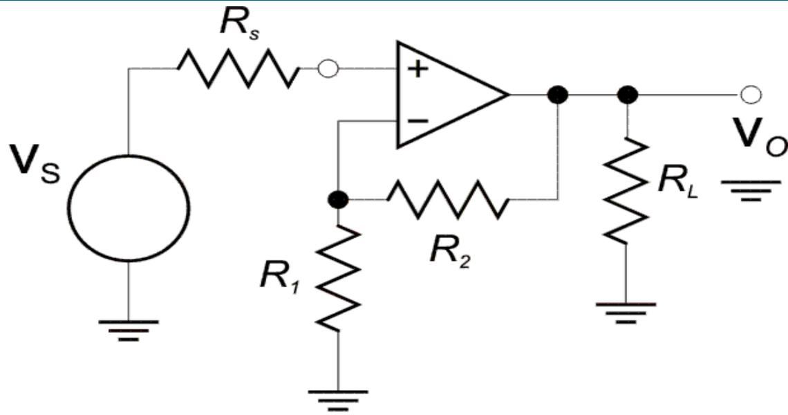
$$\beta = \frac{R_1}{R_1 + R_2}$$
