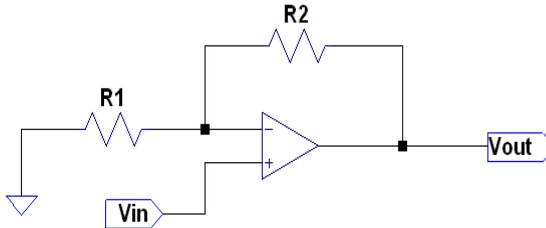
$$V_{in} \left(1 + \frac{R_2}{R_1}\right) = V_{out}$$
