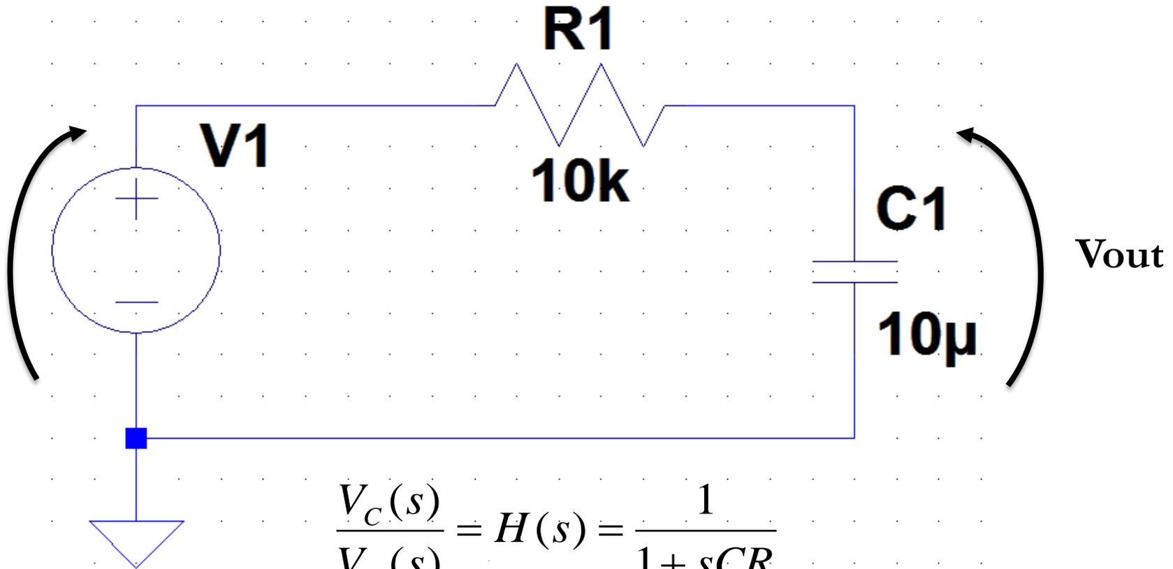
$$\frac{V_C(s)}{V_{in}(s)} = H(s) = \frac{1}{1 + sCR}$$
