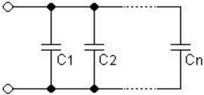
$$C_{eq} = C_1 + C_2 + C_3 + \dots + C_n$$
