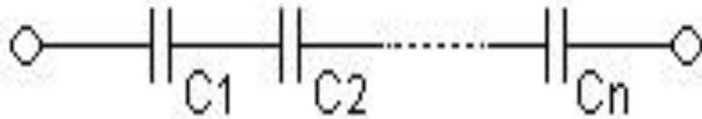
$$\frac{1}{C_{eq}} = \frac{1}{C_1} + \frac{1}{C_2} + \dots + \frac{1}{C_n}$$
