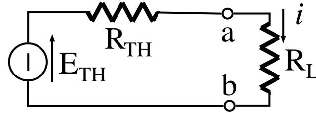
$$p = R_L i^2 = R_L \cdot \left( \frac{E_{TH}}{R_{TH} + R_L} \right)^2$$
