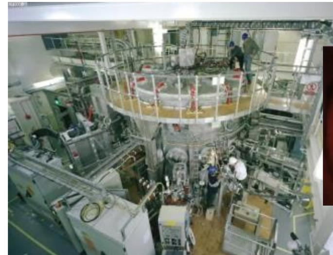
MAST spherical tokamak
