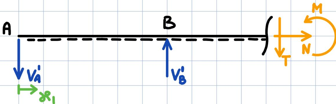
$$\bullet N'_{BC} = \emptyset \quad \bullet T'_{BC} = -V_A + V_B = 1N$$
