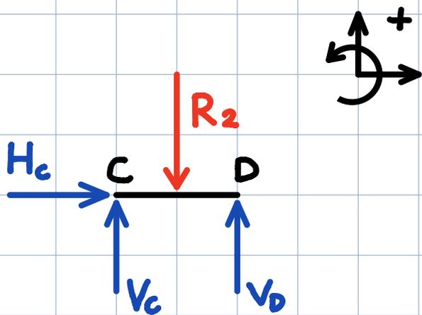
$$\begin{aligned} H_c &= 0 \\ V_c + V_d &= R_2 \\ V_d L_{CD} - R_2 \frac{L_{CD}}{2} &= 0 \end{aligned}$$
