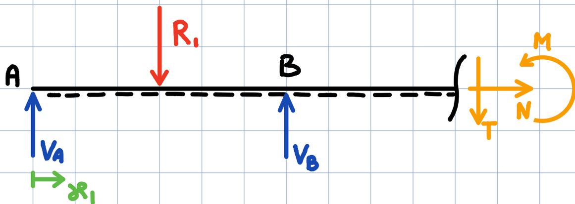
•  $N_{BC} = \emptyset$       •  $T_{BC} = V_A - \overbrace{q_1 L_{AB}}^{R_1} + V_B = 50N$
