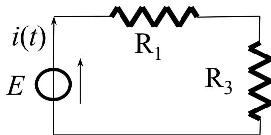
$$i(t) = I_0 = \frac{E}{R_1 + R_3} = \frac{10}{5} = 2 \text{ A}$$
