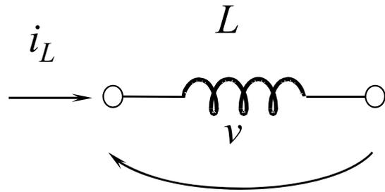
$$i_L(t) = \int_0^t \frac{1}{L} v(\tau) d\tau + \text{cost} \quad i_L(t) = \frac{\varphi(t)}{L}$$
