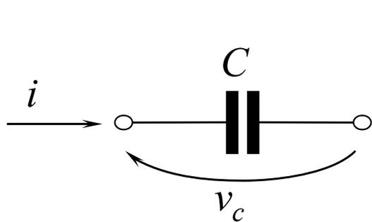
$$v_c(t) = \int_0^t \frac{1}{C} i(\tau) d\tau + \text{cost} \quad v_c(t) = \frac{q(t)}{C}$$
