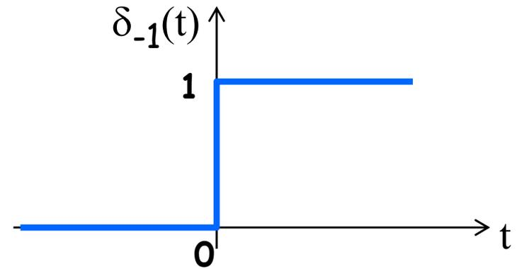
$$\delta_{-1}(t) = \begin{cases} 0 & \text{per } t < 0 \\ \text{indefinita} & \text{per } t = 0 \\ 1 & \text{per } t > 0 \end{cases}$$
