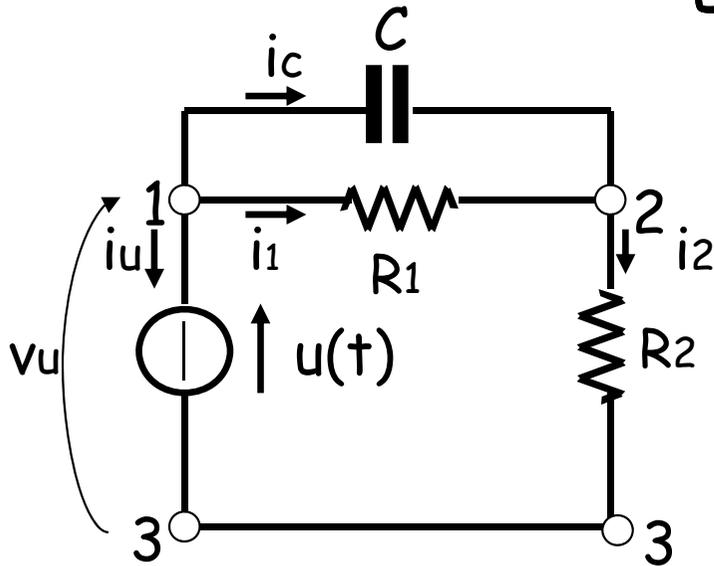
$$v_{c1}(t) = \frac{ER_1}{R_1 + R_2} \left( 1 - e^{-\frac{R_1 + R_2}{R_1 R_2 C} t} \right) \delta_{-1}(t) \text{ per } u_1(t) = E \delta_{-1}(t)$$
