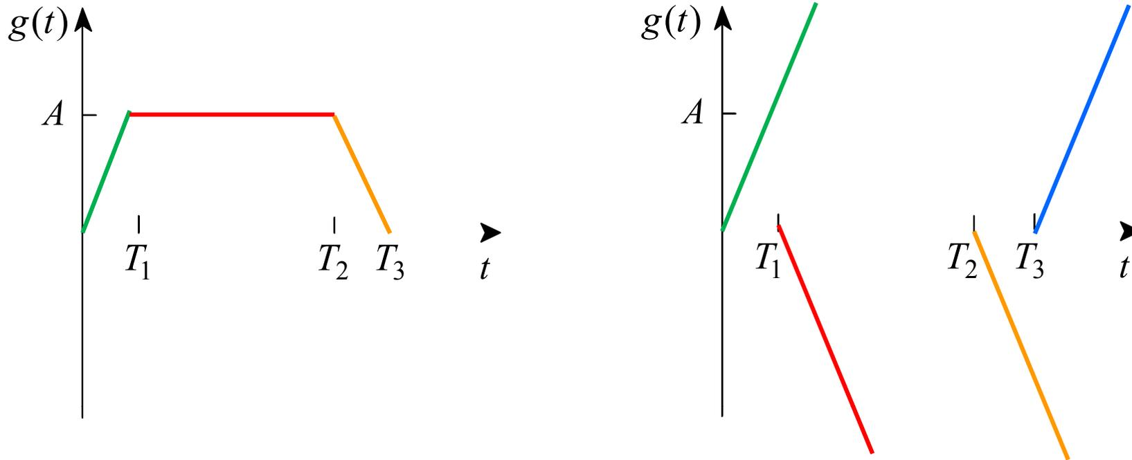
$$g(t) = \frac{A}{T_1} t \delta_{-1}(t) - \frac{A}{T_1} (t - T_1) \delta_{-1}(t - T_1) - \frac{A}{T_3 - T_2} (t - T_2) \delta_{-1}(t - T_2) + \frac{A}{T_3 - T_2} (t - T_3) \delta_{-1}(t - T_3)$$
