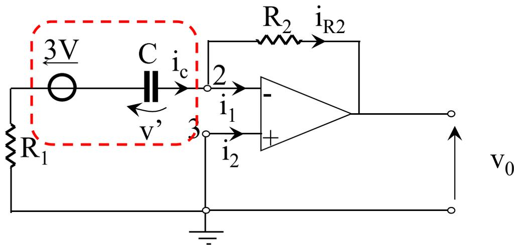
$$v_2 = v_3$$
