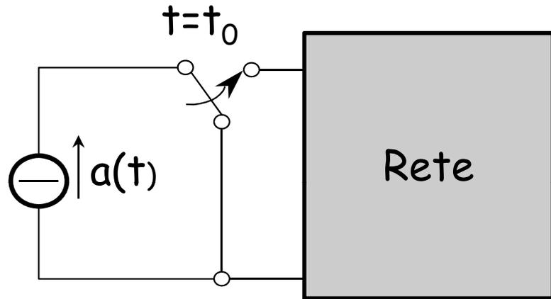
$$\delta_{-1}(t-t_0) = \begin{cases} 0 & \text{per } t < t_0 \\ 1 & \text{per } t > t_0 \end{cases}$$
