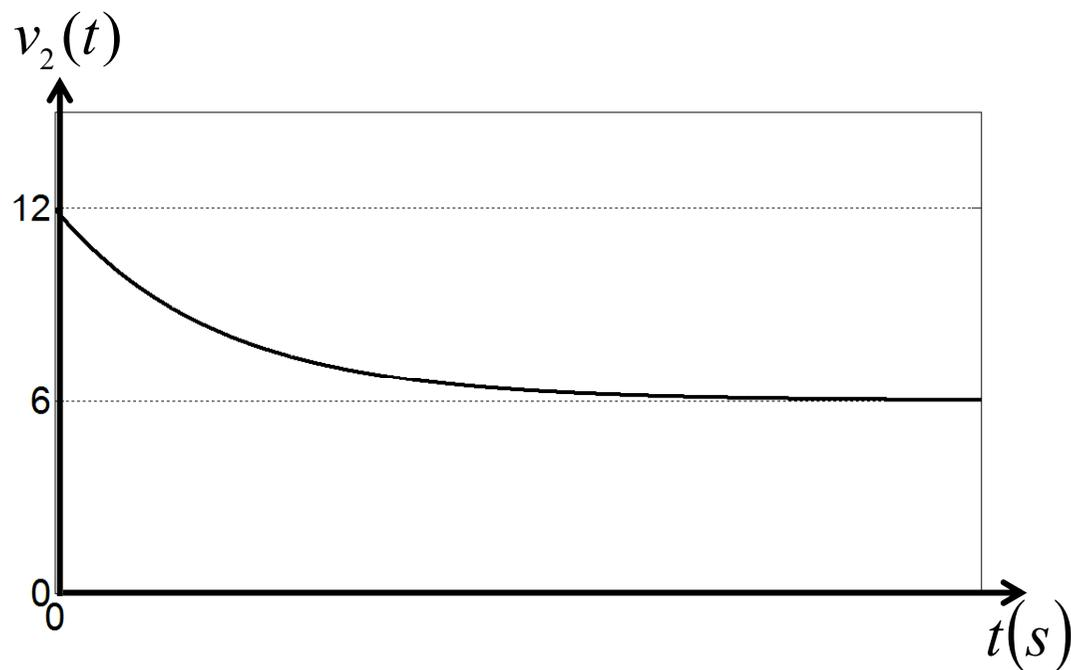
$$t = 0 \quad v_2(t) = E = 12V$$
