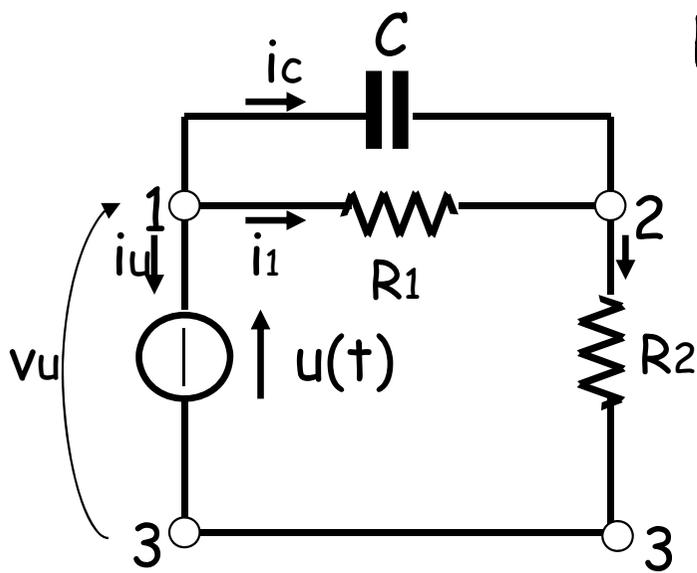
$$v_c(t) = \frac{ER_1}{R_1 + R_2} \left( 1 - e^{-\frac{R_1 + R_2}{R_1 R_2 C} t} \right) \delta_{-1}(t) \text{ per } u_1(t) = E \delta_{-1}(t)$$
