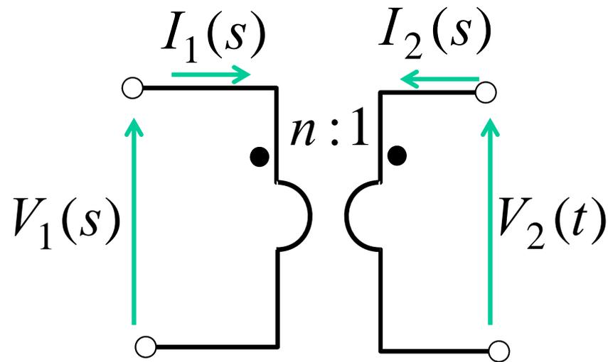
$$\begin{cases} V_1(s) = n \cdot V_2(s) \\ I_1(s) = -\frac{1}{n} \cdot I_2(s) \end{cases}$$
