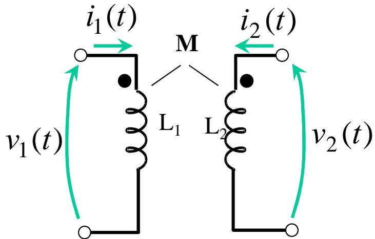
$$\begin{cases} v_1(t) = L_1 \cdot \frac{di_1}{dt} + M \cdot \frac{di_2}{dt} \\ v_2(t) = M \cdot \frac{di_1}{dt} + L_2 \cdot \frac{di_2}{dt} \end{cases} \quad \begin{aligned} i_1(0^-) \neq 0 = I_{10} \\ i_2(0^-) \neq 0 = I_{20} \end{aligned}$$
