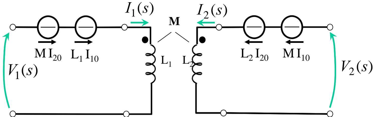
$$\begin{cases} V_1(s) = sL_1 I_1(s) + sM I_2(s) - L_1 I_{10} - M I_{20} \\ V_2(s) = sM I_1(s) + sL_2 I_2(s) - L_2 I_{20} - M I_{10} \end{cases}$$
