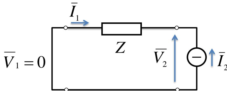
$$\begin{aligned} \bar{V}_2 &= \dot{Z} \bar{I}_2 \\ \bar{I}_1 &= -\bar{I}_2 \end{aligned} \quad \Rightarrow \quad g_{12} = \left. \frac{\bar{I}_1}{\bar{I}_2} \right|_{\bar{V}_1=0} = -1 \quad g_{22} = \left. \frac{\bar{V}_2}{\bar{I}_2} \right|_{\bar{V}_1=0} = \dot{Z}$$
