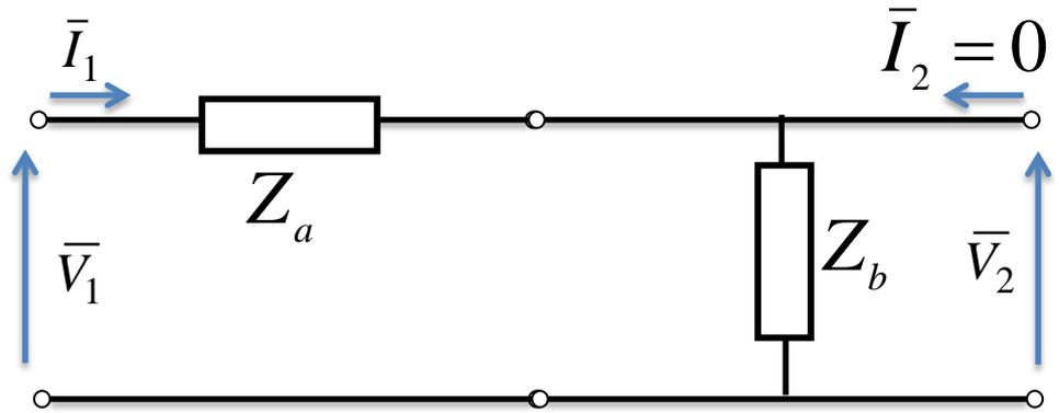
$$\bar{V}_2 = \bar{V}_1 \frac{\dot{Z}_b}{\dot{Z}_a + \dot{Z}_b} \Rightarrow \bar{V}_1 = \bar{V}_2 \frac{\dot{Z}_a + \dot{Z}_b}{\dot{Z}_b}$$
