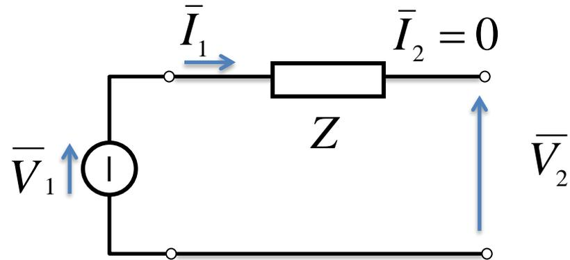
$$\begin{matrix} \bar{I}_1 = 0 \\ \bar{V}_2 = \bar{V}_1 \end{matrix} \quad \longrightarrow \quad g_{11} = \left. \frac{\bar{I}_1}{\bar{V}_1} \right|_{\bar{I}_2=0} = 0 \quad g_{21} = \left. \frac{\bar{V}_2}{\bar{V}_1} \right|_{\bar{I}_2=0} = 1$$
