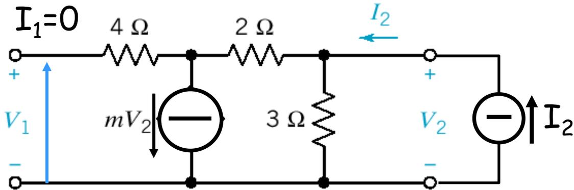
$$\begin{cases} V_2 = 3 \cdot (I_2 - mV_2) \Rightarrow V_2 + 3mV_2 = 3I_2 \Rightarrow 3 \cdot V_2 = 3I_2 \\ V_1 = V_2 - 2m\bar{V}_2 = V_2 - \frac{4}{3}V_2 = -\frac{1}{3}V_2 = -\frac{1}{3}I_2 \end{cases} \Rightarrow \begin{aligned} Z_{22} &= \left. \frac{V_2}{I_2} \right|_{I_1=0} = 1\ \Omega \\ Z_{12} &= \left. \frac{V_1}{I_2} \right|_{I_1=0} = -\frac{1}{3}\ \Omega \end{aligned}$$
