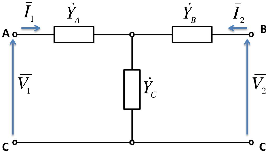
$$\dot{Y}_{11} = \left. \frac{\bar{I}_1}{\bar{V}_1} \right|_{\bar{V}_2=0} = \frac{(\dot{Y}_B + \dot{Y}_C)\dot{Y}_A}{\dot{Y}_A + \dot{Y}_B + \dot{Y}_C} = \frac{\dot{Y}_A\dot{Y}_B + \dot{Y}_C\dot{Y}_A}{\dot{Y}_A + \dot{Y}_B + \dot{Y}_C}$$
