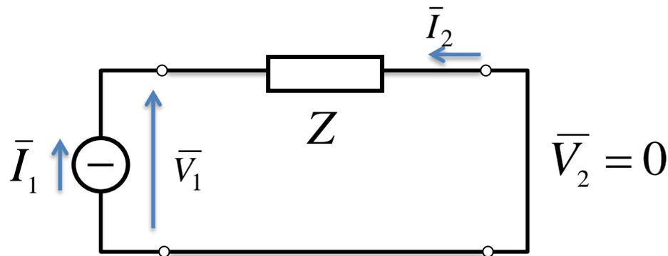
$$\begin{aligned} \bar{V}_1 &= \dot{Z} \bar{I}_1 \\ \bar{I}_2 &= -\bar{I}_1 \end{aligned} \quad \Rightarrow \quad h_{11} = \left. \frac{\bar{V}_1}{\bar{I}_1} \right|_{\bar{V}_2=0} = \dot{Z} \quad h_{21} = \left. \frac{\bar{I}_2}{\bar{I}_1} \right|_{\bar{V}_2=0} = -1$$
