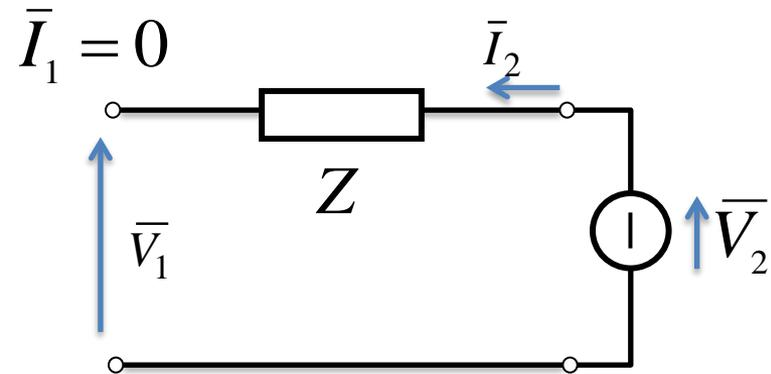
$$\begin{array}{l} \bar{V}_1 = \bar{V}_2 \\ \bar{I}_2 = 0 \end{array} \quad \Rightarrow \quad h_{12} = \left. \frac{\bar{V}_1}{\bar{V}_2} \right|_{\bar{I}_1=0} = 1 \quad h_{22} = \left. \frac{\bar{I}_2}{\bar{V}_2} \right|_{\bar{I}_1=0} = 0$$
