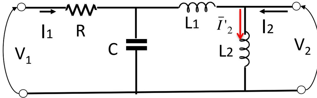
$$\begin{cases} \bar{V}_1 = \dot{Z}_{11} \bar{I}_1 + \dot{Z}_{12} \bar{I}_2 \\ \bar{V}_2 = \dot{Z}_{21} \bar{I}_1 + \dot{Z}_{22} \bar{I}_2 \end{cases}$$
