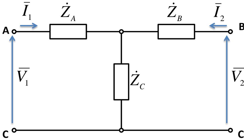
$$[\dot{Z}] = \begin{bmatrix} \dot{Z}_A + \dot{Z}_C & \dot{Z}_C \\ \dot{Z}_C & \dot{Z}_B + \dot{Z}_C \end{bmatrix}$$
