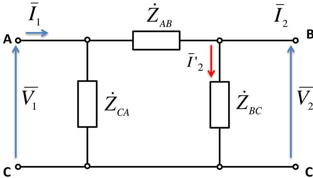
$$[\dot{Z}] = \begin{bmatrix} \frac{\dot{Z}_{AB}\dot{Z}_{CA}}{\dot{Z}_{\Delta}} + \frac{\dot{Z}_{BC}\dot{Z}_{CA}}{\dot{Z}_{\Delta}} & \frac{\dot{Z}_{BC}\dot{Z}_{CA}}{\dot{Z}_{\Delta}} \\ \frac{\dot{Z}_{BC}\dot{Z}_{CA}}{\dot{Z}_{\Delta}} & \frac{\dot{Z}_{AB}\dot{Z}_{BC}}{\dot{Z}_{\Delta}} + \frac{\dot{Z}_{BC}\dot{Z}_{CA}}{\dot{Z}_{\Delta}} \end{bmatrix}$$
