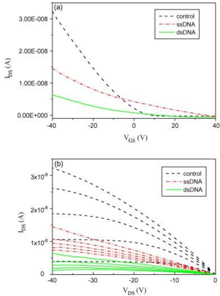
Label-free DNA sensor based on organic thin film transistors
