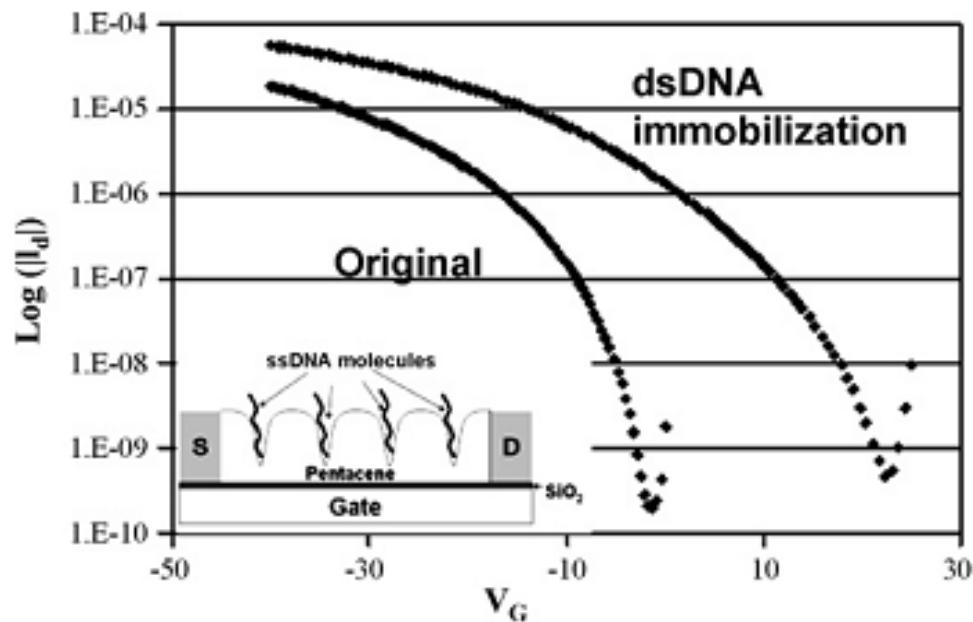
DNA hybridization detection with organic thin film transistors:
