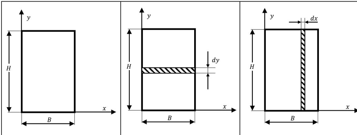
$$x_G = \frac{\int_A x dA}{A} \quad \text{Poiché: } dA = H dx \text{ da cui: } x_G = \frac{H \int_0^B x dx}{BH} = \frac{x^2|_0^B}{2B} = \frac{B}{2}$$
