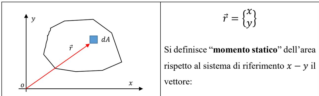
$$\vec{S} = \int_A \vec{r} dA = \begin{Bmatrix} \int_A x dA \\ \int_A y dA \end{Bmatrix} = \begin{Bmatrix} S_y \\ S_x \end{Bmatrix} \quad (1)$$
