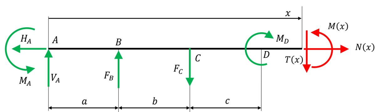
$$\left\{ \begin{aligned} \sum F_x &= N(x) - H_A = 0 \\ \sum F_y &= V_A + F_B - F_C - T(x) = 0 \\ \sum_x M_z &= M(x) + M_A - V_A x - F_B(x - a) - F_C[x - (a + b)] - M_D = 0 \end{aligned} \right.$$
