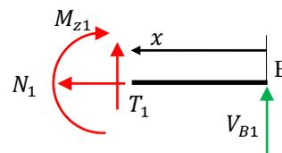
$$\begin{cases} \sum F_{\parallel} = N_1(x) = 0 \\ \sum F_{\perp} = T_1(x) + V_{B1} = 0 \\ \sum M = M_{z1}(x) - V_{B1}x = 0 \end{cases}$$
