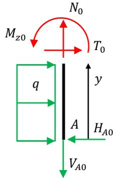
$$\begin{cases} \sum F_{\parallel} = N_0(y) - V_{A0} = 0 \\ \sum F_{\perp} = T_0(y) + qy - H_{A0} = 0 \\ \sum M = M_{z0}(y) + \frac{qy^2}{2} - H_{A0}y = 0 \end{cases}$$
