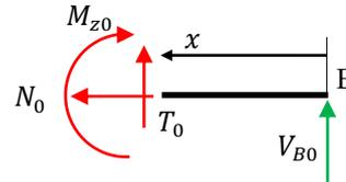
$$\begin{cases} \sum F_{\parallel} = N_0(x) = 0 \\ \sum F_{\perp} = T_0(x) + V_{B0} = 0 \\ \sum M = M_{z0}(x) - V_{B0}x = 0 \end{cases}$$
