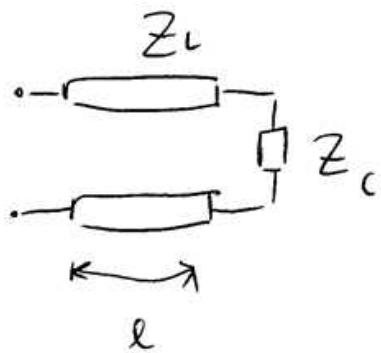
$$Y_{IN} = \frac{1}{Z_L} \cdot \frac{\frac{1}{Z_C} + j \frac{1}{Z_L} t_p(\beta l)}{\frac{1}{Z_L} + j \frac{1}{Z_C} t_p(\beta l)}$$
