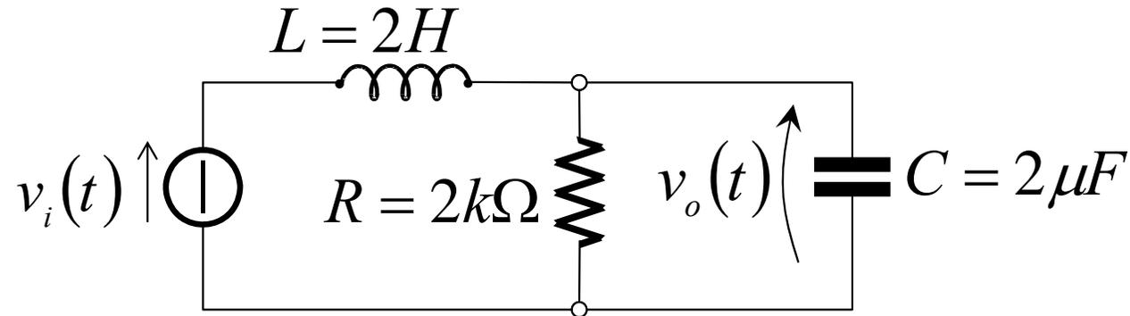
$$|\dot{H}(j\omega)| = \frac{R}{\sqrt{(R - \omega^2 RLC)^2 + (\omega L)^2}} = \frac{1}{\sqrt{2}} \Rightarrow \frac{R^2}{(R - \omega^2 RLC)^2 + (\omega L)^2} = \frac{1}{2}$$
