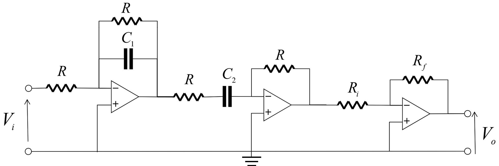
$$\Rightarrow \text{scegliendo } R_i = 10k\Omega \quad \Rightarrow R_f = 10.83 R_i \cong 108k\Omega$$
