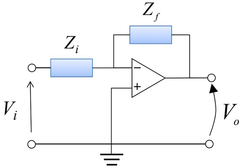
$$\dot{H}(j\omega) = \frac{\bar{V}_o}{\bar{V}_i} = -\frac{\dot{Z}_f}{\dot{Z}_i}$$
