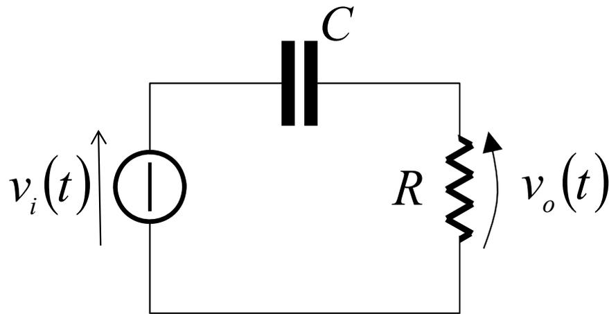
$$\dot{H}(\omega) = \frac{\overline{V_o}}{\overline{V_s}} = \frac{R}{R + \frac{1}{j\omega C}} = \frac{j\omega R C}{1 + j\omega R C} \quad \text{ponendo} \quad \omega_0 = \frac{1}{RC}$$
