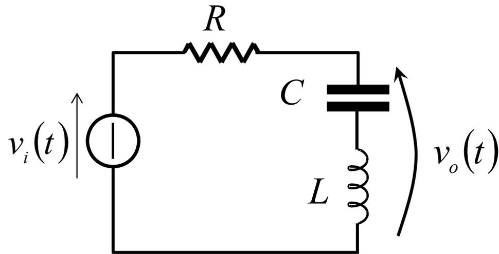
$$\dot{H}(j\omega) = \frac{\bar{V}_0}{\bar{V}_i} = \frac{j\left(\omega L - \frac{1}{\omega C}\right)}{R + j\left(\omega L - \frac{1}{\omega C}\right)}$$
