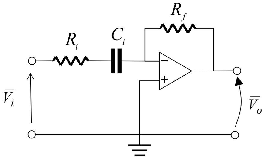
$$\dot{H}(j\omega) = \frac{\bar{V}_o}{\bar{V}_i} = -\frac{\dot{Z}_f}{\dot{Z}_i}$$
