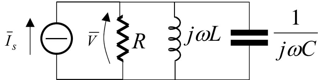
$$\dot{H}(j\omega) = \dot{Z} = \frac{\bar{V}}{\bar{I}_s} = \frac{1}{\dot{Y}} = \frac{1}{\frac{1}{R} + \frac{1}{j\omega L} + j\omega C} = \frac{1}{\frac{1}{R} + j\left(\omega C - \frac{1}{\omega L}\right)}$$
