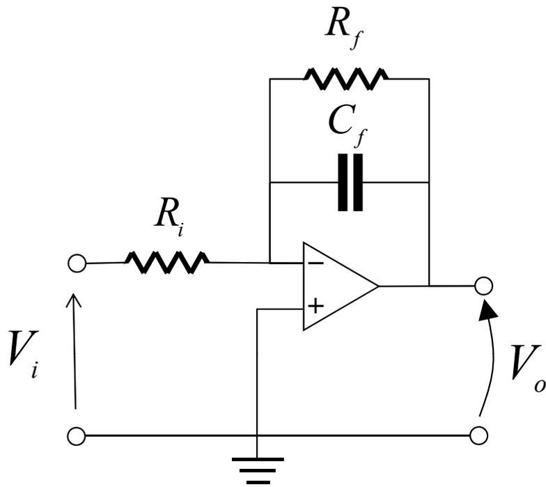
$$\left\{ \begin{array}{l} \omega_c = \frac{1}{R_f C_f} = 2\pi \cdot 500 \\ H(0) = -\frac{R_f}{R_i} = -4 \end{array} \right.$$
