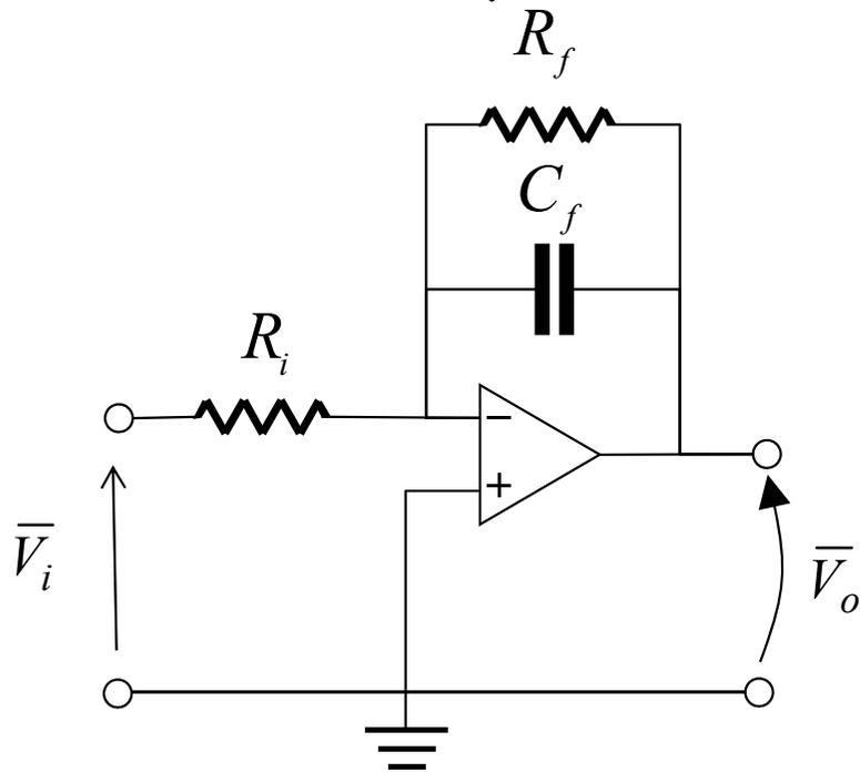
$$\dot{Z}_i = R_i \quad \dot{Z}_f = R_f \parallel \frac{1}{j\omega C_f} = \frac{R_f \cdot \frac{1}{j\omega C_f}}{R_f + \frac{1}{j\omega C_f}} = \frac{R_f}{1 + j\omega R_f C_f}$$
