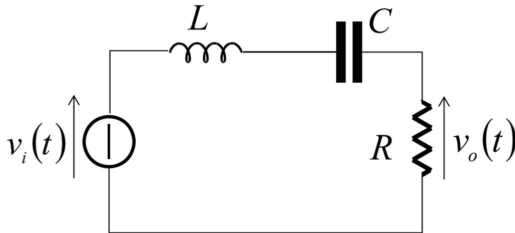
$$H(j\omega) = \frac{V_o}{V_i} = \frac{R}{R + j\left(\omega L - \frac{1}{\omega C}\right)}$$
