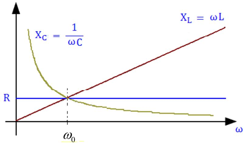
per  $\omega = \omega_0 = \frac{1}{\sqrt{LC}} \quad |Z| = R \quad \varphi = 0$
