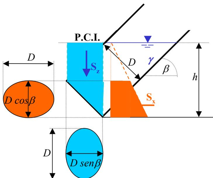
$$\left[ \begin{array}{l} S = \gamma [h - (D/2) \cos \beta] \pi D^2 / 4 = 17475 \text{ N} \\ S_x = \gamma [h - (D/2) \cos \beta] \pi (D/2) (D \cos \beta / 2) = 12357 \text{ N} \leftarrow \\ S_z = \gamma \pi (D/2) (D \sin \beta / 2) [h - (D/2) \cos \beta] = 12357 \text{ N} \downarrow \\ \xi = [h / \cos \beta - (D/2)] + 1/16 D^2 [h / \cos \beta - (D/2)] = 2,269 \text{ m} \end{array} \right.$$
