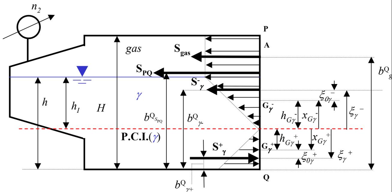
$$\left[ \begin{array}{lll} S_{gas} = -5000 \text{ N, applicata in } [H-h]/2 & S_\gamma^+ = 1131 \text{ N} & \xi_\gamma^+ = 0,320 \text{ m} \\ S_\gamma^- = -5099 \text{ N} & \xi_\gamma^- = -0,680 \text{ m} & S = S_\gamma^+ - |S_{gas}| - |S_\gamma^-| = -8968 \text{ N} \\ & & b_{sPQ}^Q = 1,615 \text{ m} \end{array} \right]$$
