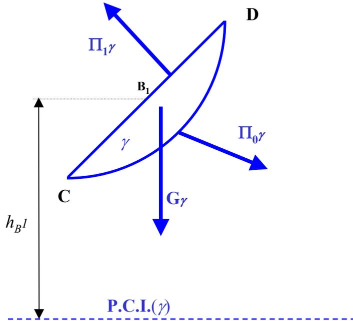
$$\left[ \begin{array}{l} S_{CDx} = \gamma h_{B1} R L = 139619 \text{ N} \quad \leftarrow \\ S_{CDz} = |\gamma h_{B1} R L - \gamma [1/4 \pi R^2 - 1/2 R^2] L| = 114935 \text{ N} \quad \uparrow \end{array} \right]$$
