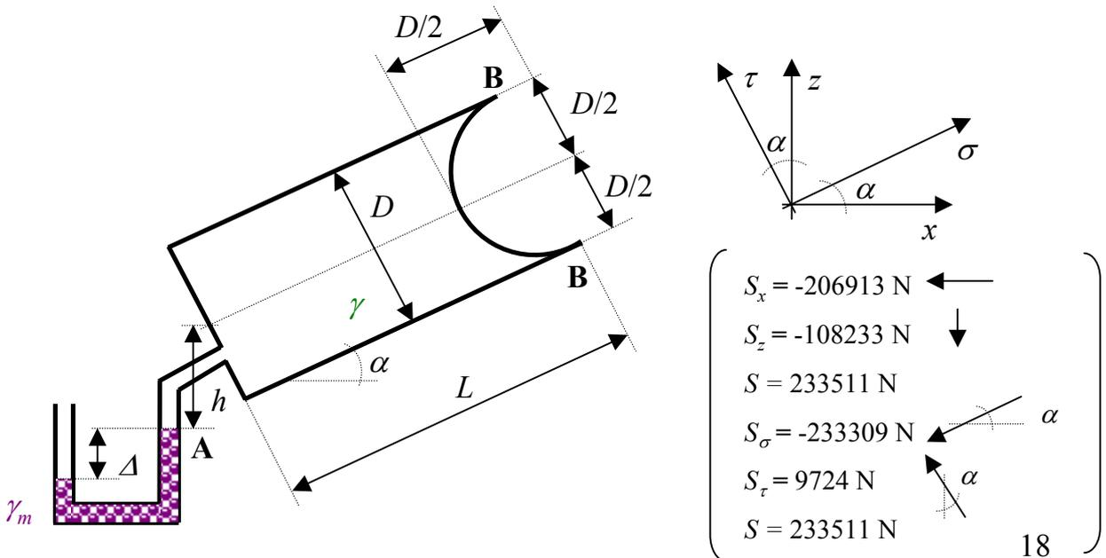
$$\left( \begin{array}{lll} S_x = -206913 \text{ N} \longleftarrow & & \\ S_z = -108233 \text{ N} \downarrow & & \\ S = 233511 \text{ N} & & \\ S_\sigma = -233309 \text{ N} \nwarrow \alpha & & \\ S_\tau = 9724 \text{ N} \nwarrow \alpha & & \\ S = 233511 \text{ N} & & \end{array} \right) \quad 18$$
