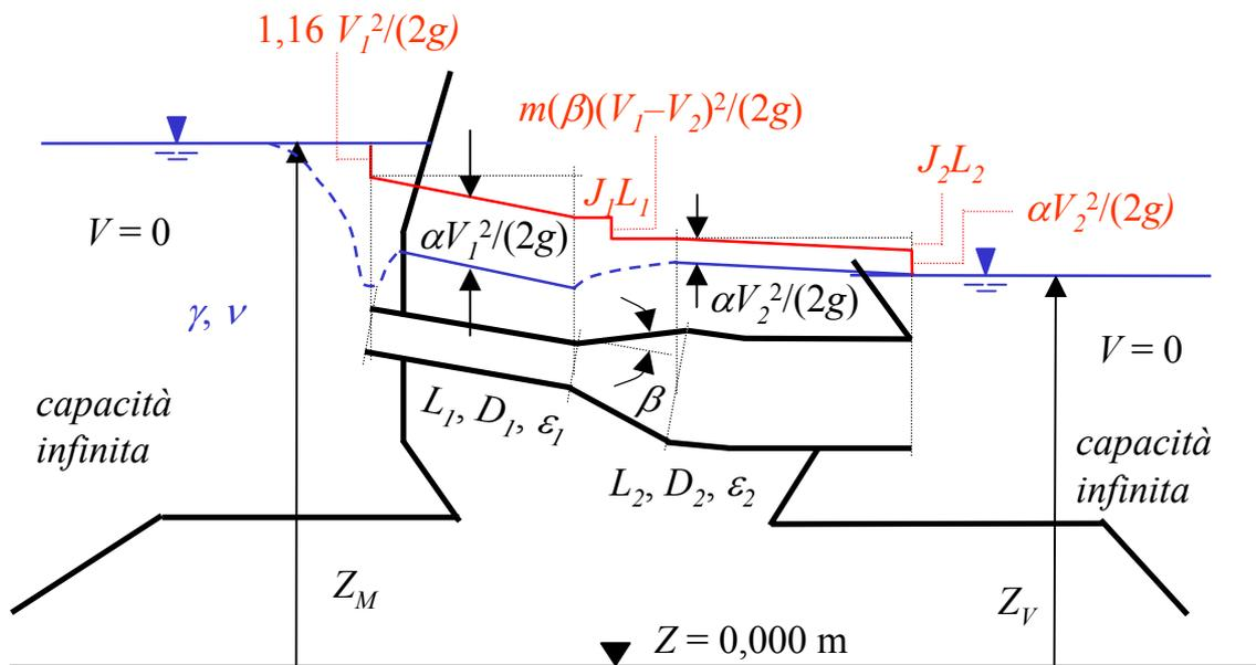
$$\left[ \begin{aligned} Z_M &= 1,16 V_1^2/(2g) + J_{1,1} L_1 + m(\beta) (V_1 - V_2)^2/(2g) + J_2 L_2 + \alpha V_2^2/(2g) + Z_V = 32,713 \text{ m} \\ Z_M &= 1,16 V_1^2/(2g) + J_{1,2} L_1 + m(\beta) (V_1 - V_2)^2/(2g) + J_2 L_2 + \alpha V_2^2/(2g) + Z_V = 33,375 \text{ m} \end{aligned} \right]$$
