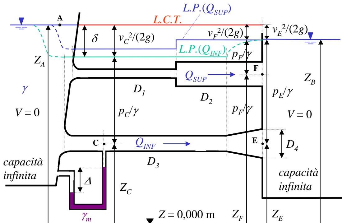
$$\left[ \begin{array}{l} Q_{INF} = A_3 [2 g \Delta (\gamma_m - \gamma) / \gamma]^{1/2} = 0,125 \text{ m}^3/\text{s} \quad Z_B = Z_A - Q_{INF}^2 / (2 g A_4^2) = 20,841 \text{ m} \\ Q_{SUP} = A_2 [2 g (Z_A - Z_B)]^{1/2} = 0,087 \text{ m}^3/\text{s} \end{array} \right]$$
