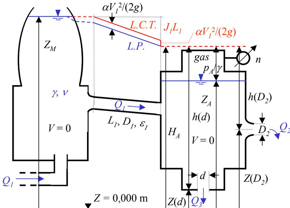
$$\left[ \begin{array}{l} Q_2 = \mu(D_2) A(D_2) [2 g h(D_2)]^{1/2} = 0,403 \text{ m}^3/\text{s} \\ Q_3 = \mu(d) A(d) [2 g h(d)]^{1/2} = 0,154 \text{ m}^3/\text{s} \\ Q_1 = Q_2 + Q_3 = 0,557 \text{ m}^3/\text{s} \\ Z_M = \alpha V_1^2 / (2 g) + J_1 L_1 + H_A = 14,838 \text{ m} \end{array} \right]$$
