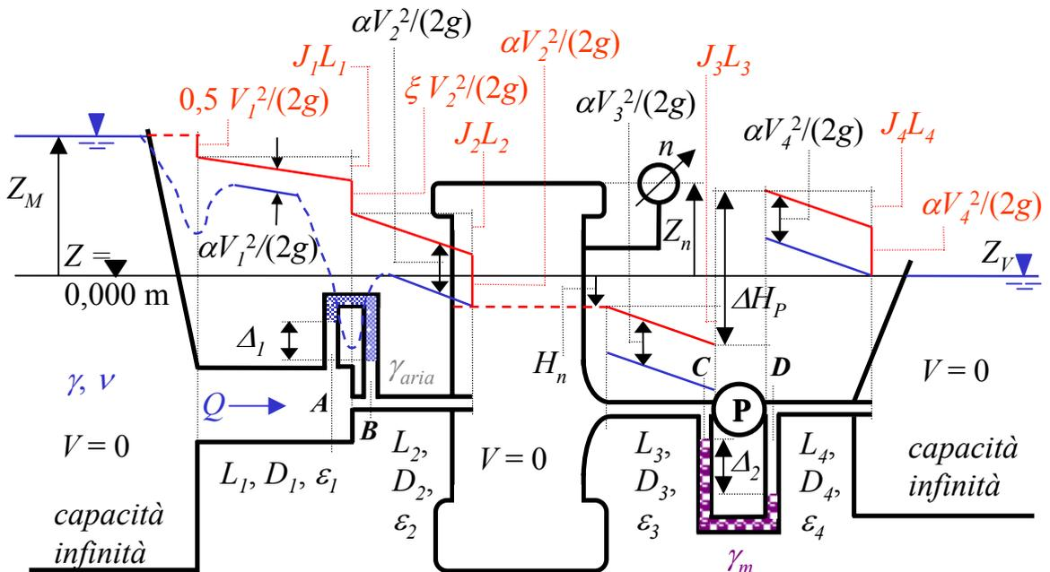
$$Q = \{ [2 g \Delta_1 / [(1 + \xi) A_2^2 - 1/A_1^2]] \}^{1/2} = 0,275 \text{ m}^3/\text{s} \quad \Delta H_P = \Delta_2 (\gamma_m - \gamma) / \gamma = 3,200 \text{ m}$$
