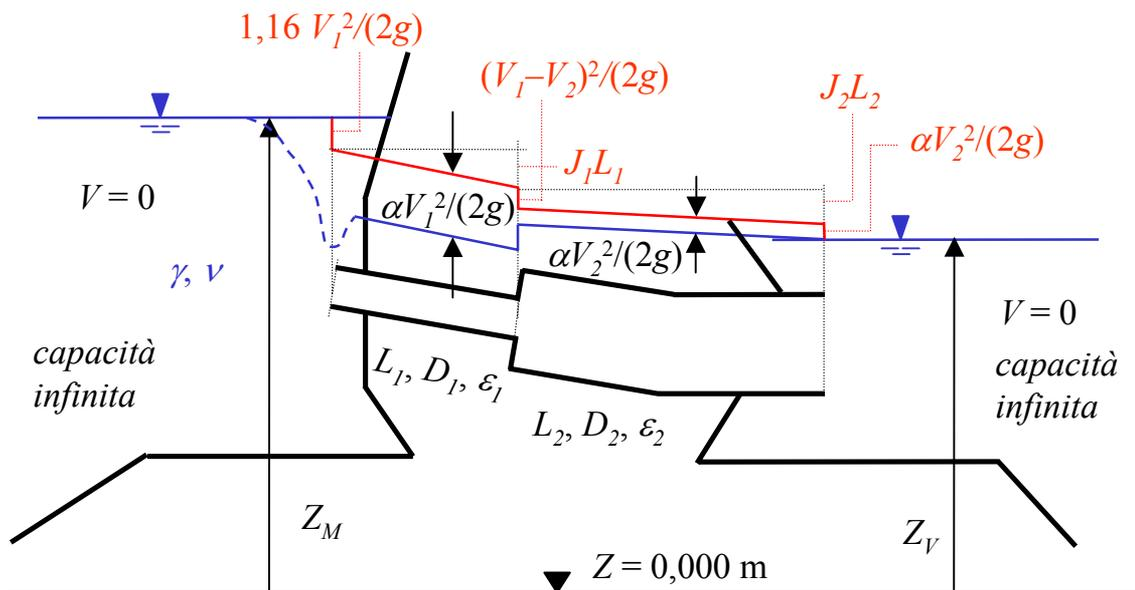
$$\left[ \begin{aligned} Z_M &= 1,16 V_1^2/(2g) + J_{1,1} L_1 + (V_1 - V_2)^2/(2g) + J_2 L_2 + \alpha V_2^2/(2g) + Z_V = 32,837 \text{ m} \\ Z_M &= 1,16 V_1^2/(2g) + J_{1,2} L_1 + (V_1 - V_2)^2/(2g) + J_2 L_2 + \alpha V_2^2/(2g) + Z_V = 33,498 \text{ m} \end{aligned} \right]$$
