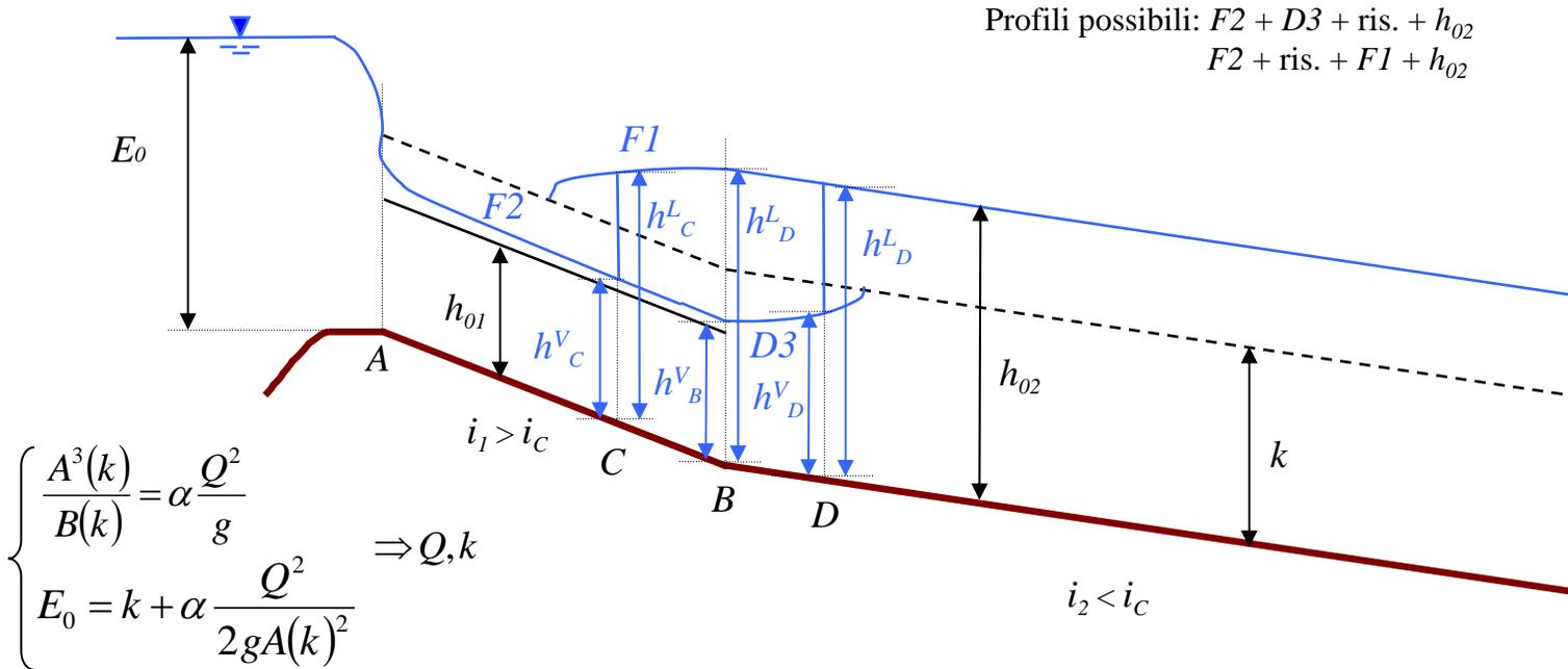
$$S(h_B^V) = \gamma \langle h_B^V \rangle_G A(h_B^V) + \beta \rho \frac{Q^2}{A(h_B^V)} > \gamma \langle h_B^L \rangle_G A(h_B^L) + \beta \rho \frac{Q^2}{A(h_B^L)} = S(h_B^L) \Rightarrow$$
