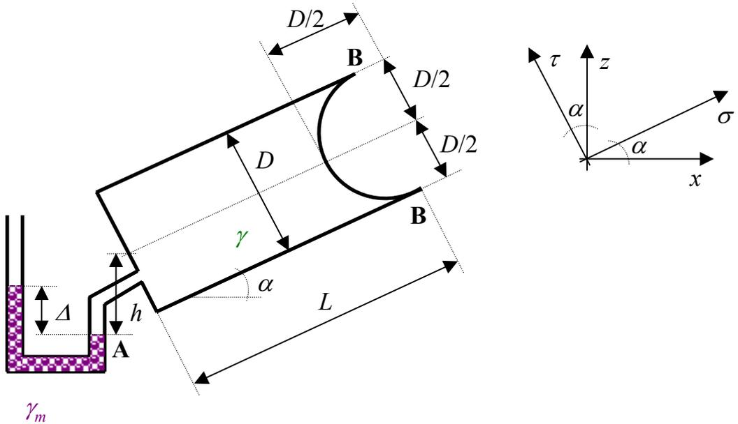
$$\left( \begin{array}{lll} S_x = 86985 \text{ N} \longrightarrow & S_z = 61449 \text{ N} \uparrow & S = 106501 \text{ N} \\ S_\sigma = 106056 \text{ N} \nearrow \alpha & S_\tau = 9724 \text{ N} \nearrow \alpha & S = 106501 \text{ N} \end{array} \right)$$
