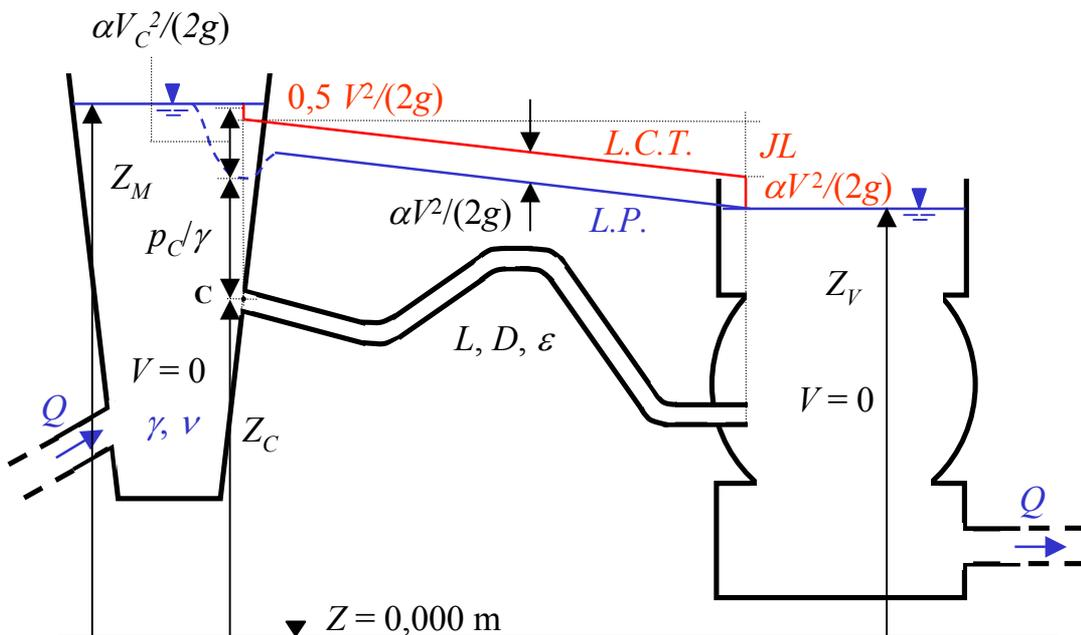
$$\left[ \begin{aligned} Q^{(IV)} &= A \{ [2g(Z_M - Z_V)] / [0,5 + \lambda^{(III)} L/D + 1] \}^{1/2} = 0,0409 \text{ m}^3/\text{s} \\ p_C &= \gamma \{ Z_M - [Z_C + \alpha V_C^2 / (2g) + 0,1 V^2 / (2g)] \} = 108811 \text{ Pa} \end{aligned} \right.$$
