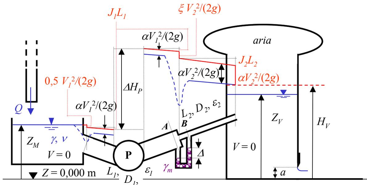
$$Q = \left\{ \frac{2g\Delta(\gamma_m - \gamma)/\gamma}{(1 + \xi)/A_2^2 - 1/A_1^2} \right\}^{1/2} = 0,288 \text{ m}^3/\text{s} \quad H_V = C_C a + \frac{Q^2}{[(\mu a b)^2 2g]} = 13,050 \text{ m}$$
