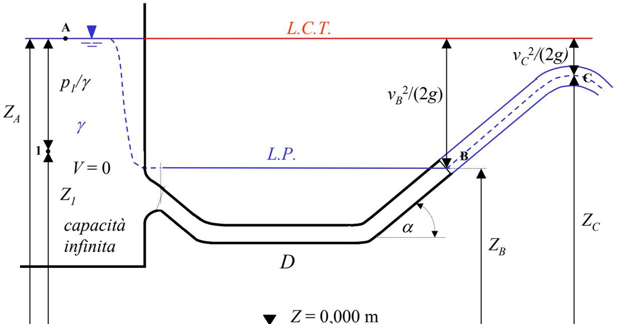
$$\left[ \begin{array}{l} Q = \pi D^2/4 [2g(Z_A - Z_B)]^{1/2} = 2,800 \text{ m}^3/\text{s} \\ Z_C(\alpha = 90^\circ) = Z_{C,MAX} = Z_A = 50,000 \text{ m} \end{array} \quad Z_C(\alpha) = Z_A - [v_B^2/(2g)] \cdot [\cos\alpha]^2 = 47,500 \text{ m} \right]$$
