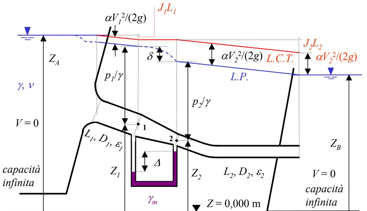
$$Q = [A_1 A_2] / [A_1^2 - A_2^2]^{1/2} [2 g \Delta (\gamma_m - \gamma) / \gamma]^{1/2} = 0,049 \text{ m}^3/\text{s}$$
