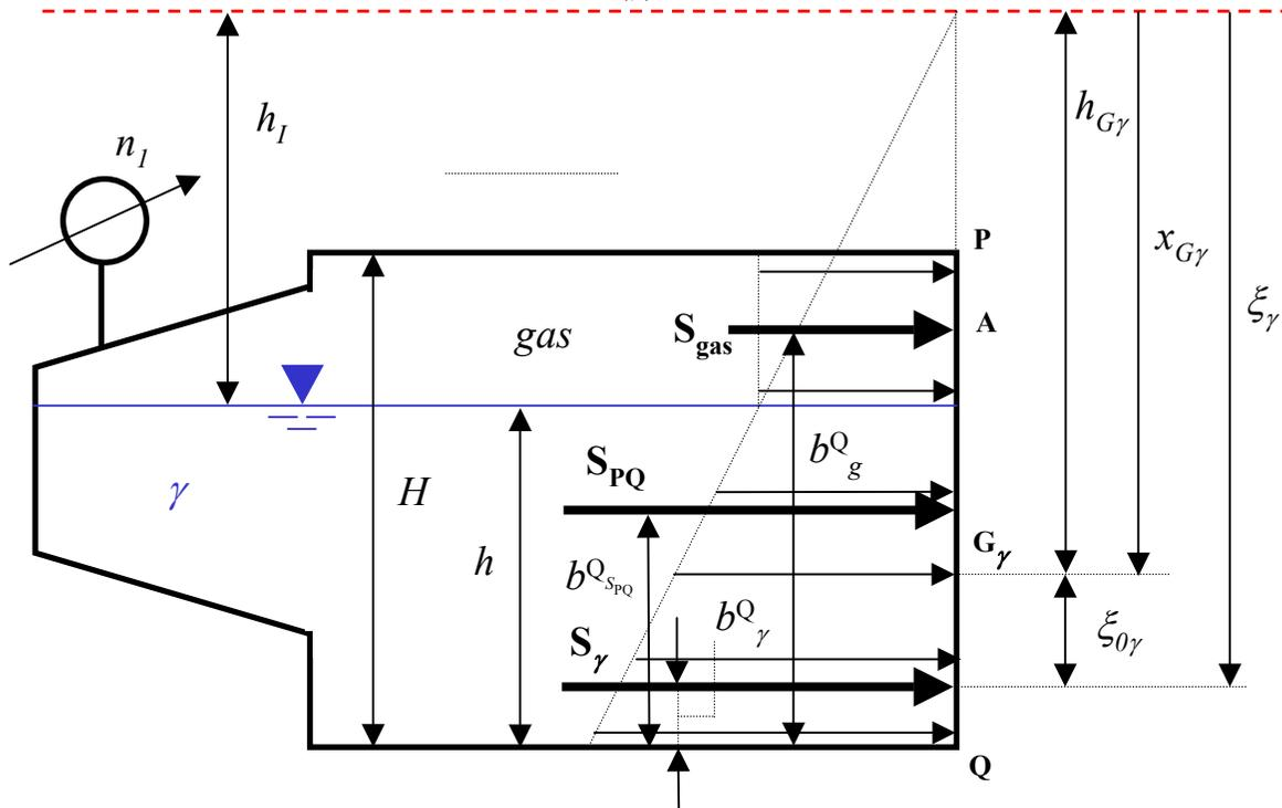
$$\left[ \begin{array}{lll} S_{gas} = 5000 \text{ N, applicata in } [H-h]/2 & S_\gamma = 26032 \text{ N} & \\ \xi_\gamma = 1,876 \text{ m} & S = S_{gas} + S_\gamma = 31032 \text{ N} & b_{sPQ}^Q = 0,882 \text{ m} \end{array} \right]$$
