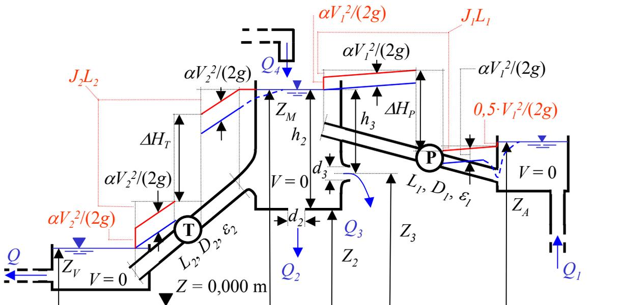
$(W_p = 389153$  W  $Q_2 = 0,066$  m<sup>3</sup>/s  $Q_3 = 0,083$  m<sup>3</sup>/s  $Q_4 = 0,551$  m<sup>3</sup>/s  $W_T = 1244567$  W) 52
