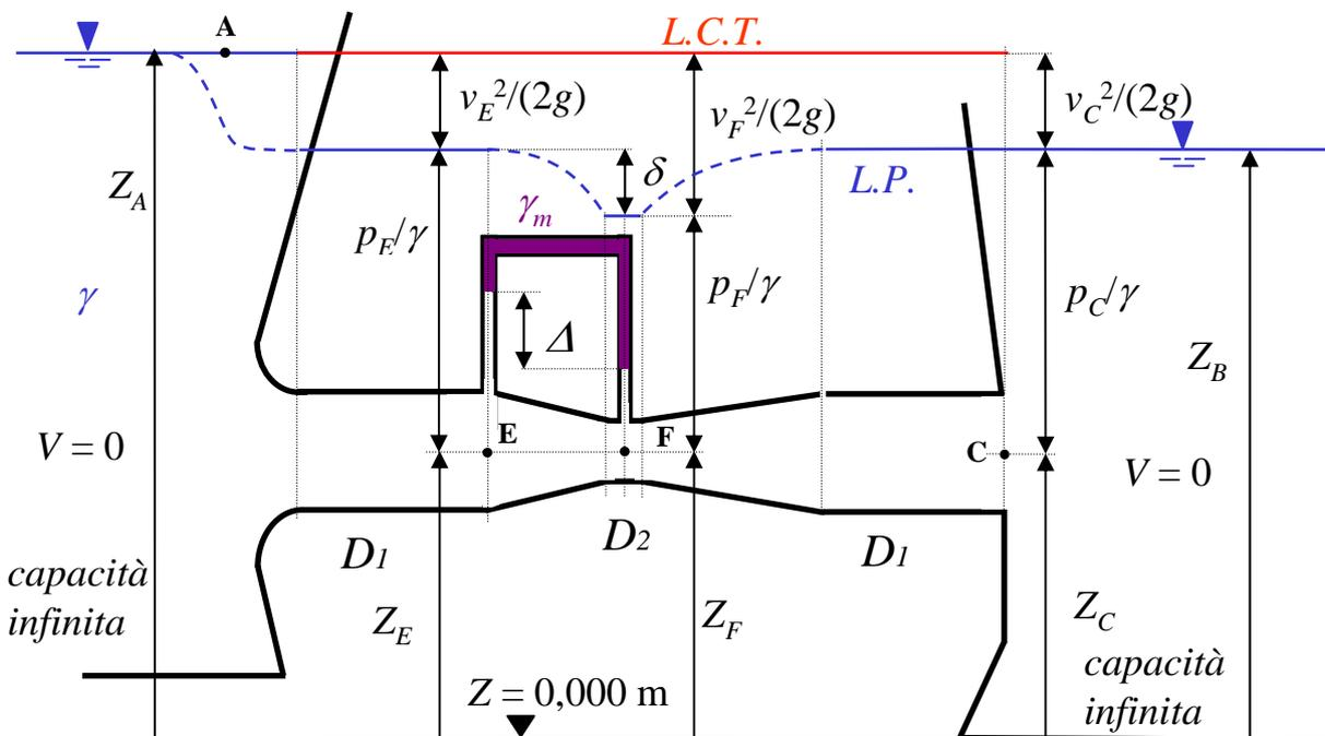
$$\left[ \begin{aligned} Q &= \pi D_1^2/4 [2 g (Z_A - Z_B)]^{1/2} = 0,870 \text{ m}^3/\text{s} \\ \Delta &= \gamma/(\gamma - \gamma_m) Q^2/(2 g) [A_1^2 - A_2^2]/[A_1^2 A_2^2] = 1,501 \text{ m} \end{aligned} \right]$$
