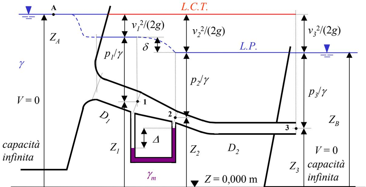
$$Q = [A_1 A_2] / [A_1^2 - A_2^2]^{1/2} [2 g \Delta (\gamma_m - \gamma) / \gamma]^{1/2} = 0,049 \text{ m}^3/\text{s}$$
