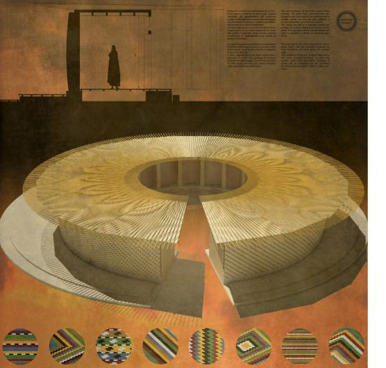
The cover - made of galvanized radial steel beams and corrugated metal sheet - is designed as a light element in contrast to the tectonic body of the earthen wall.
